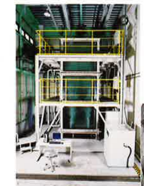
MF Membrane Unit RO Membrane Unit Wastewater recycling system with membrane technology. Sewage treatment water filtrated with membrane can be reused as industrial water.
